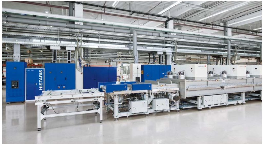
HISTARIS - Inline sputtering system with horizontal substrate transport
